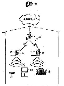
request to its own device, and turn its own device into an incoming call response and speech state when the incoming request is issued from the master telephone set, and infrared ray remote controllers 17 and 18 equipped with contact type feeding terminals which charge those slave telephone sets, which fetch audible signals from the speaker parts of the slave telephone sets, identify control information from the audible signals, and remote-control electronic equipments 19, 20, and 21.
